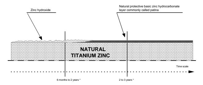
Phase one = formation of zinc hydroxide and then zinc hydroxycarbonate in the presence of relevant quantities of oxygen – contained in water- and carbon dioxide.
